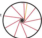
Check your work. All <u>spoke heads should be on the outside edges of the hub.</u> The holes on the rim should be a <u>right spoke</u>, <u>left spoke</u>, <u>empty</u>, <u>empty pattern</u> when viewed from the drive-side.
